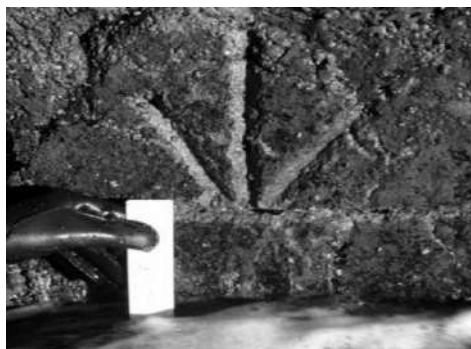
Figure 63. Zoom on the etched benchmark displayed in the ellipse (near center-left) of Figure 62, that was engraved under the order of Capt. Sir James Clark Ross in 1841 to indicate the mean sea level at the Isle of the Dead (Tasmania). After Hunter et al. (2003).
